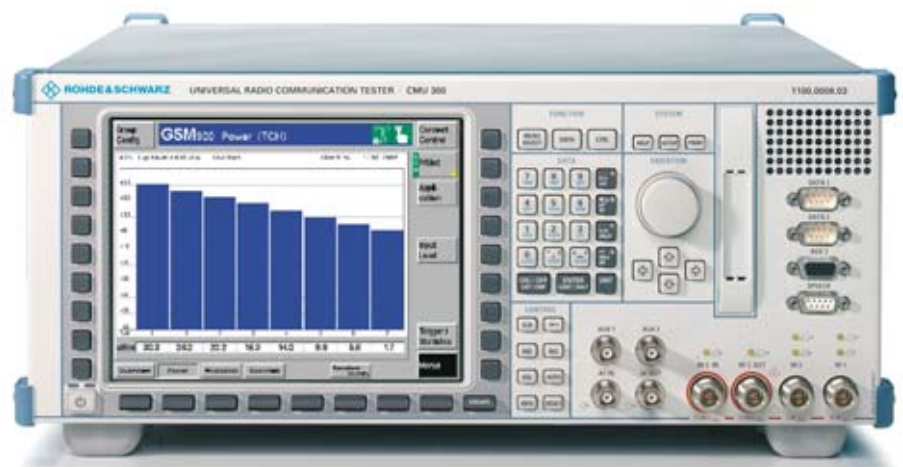
The CMU300 can handle a wide range of applications, but is primarily optimized for the high accuracy and speed demanded in an ever more quality-conscious manufacturing process. The picture shows the front panel for desktop use
