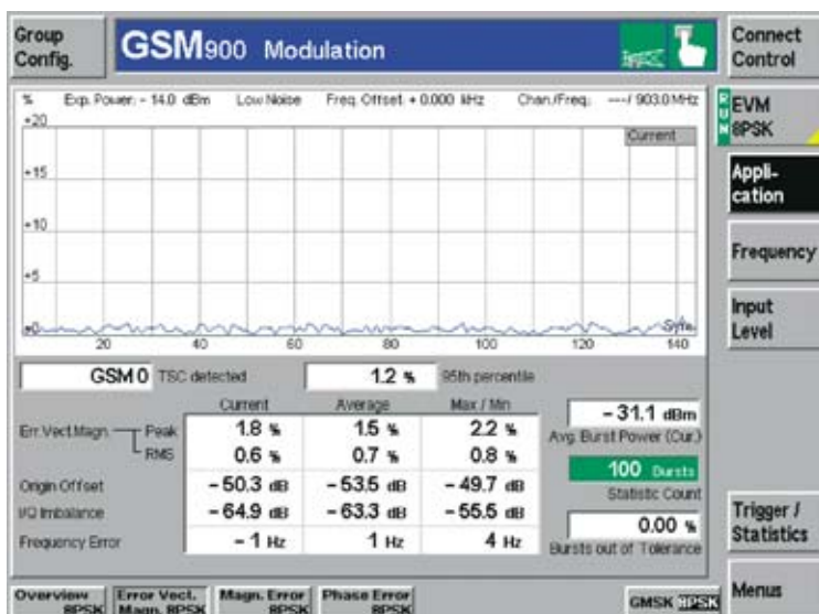
The error vector magnitude hotkey gives access to the graphical display
